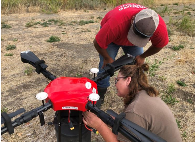
Chief Drone Pilot Anita Baumgart instructs Drone Assistant Intern Abel Rodelo how to switch out the batteries on the drone.
