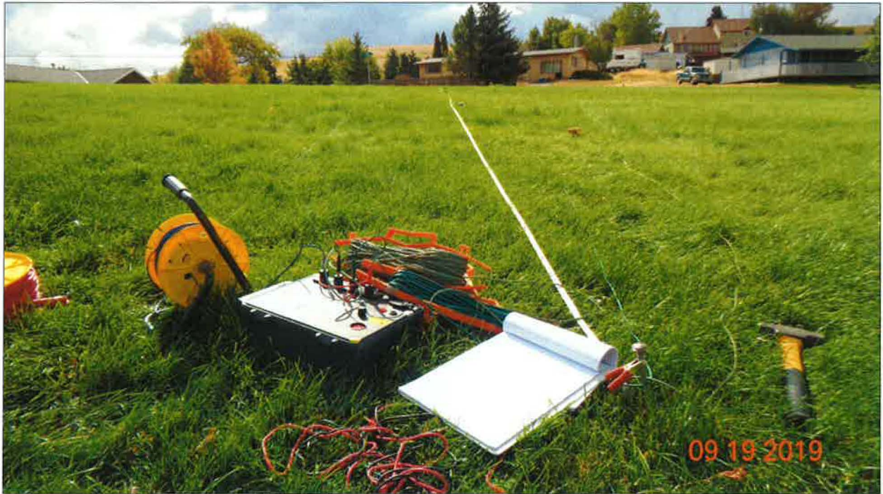
Photo 3: Soil Resistivity Test
