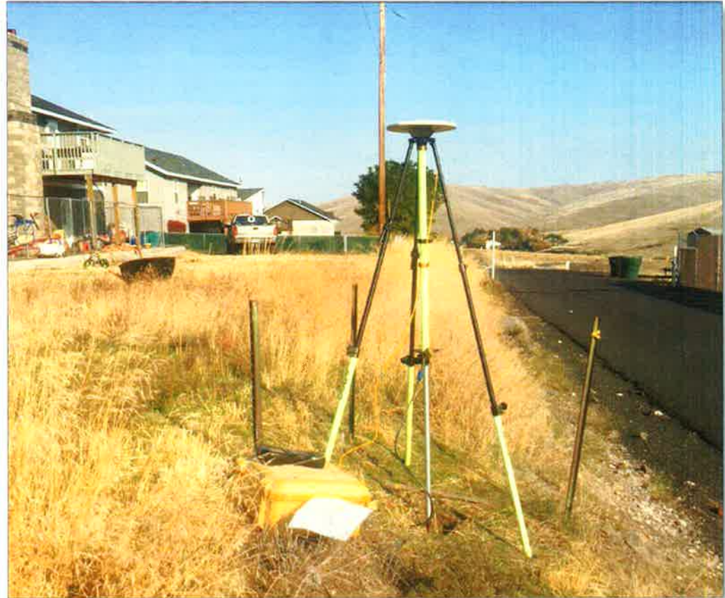
Figure 2: Zephyr GNSS Geodetic Model 2 antenna set up over RB1491 monument
